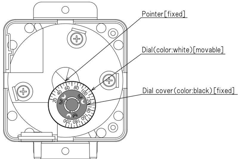
Set the tip of the pointer to the pressure you desire by knobbing the outer periphery of the dial to rotate the dial. Turning the pointer from the lower side (anti-clockwise) is recommended to set accurately with good reproducibility. Turning the pointer from the lower side (anti-clockwise) is recommended to set accurately with good reproducibility.
