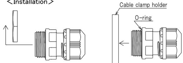
1. Remove the locknut. The locknut is not necessary to install the instrument.
